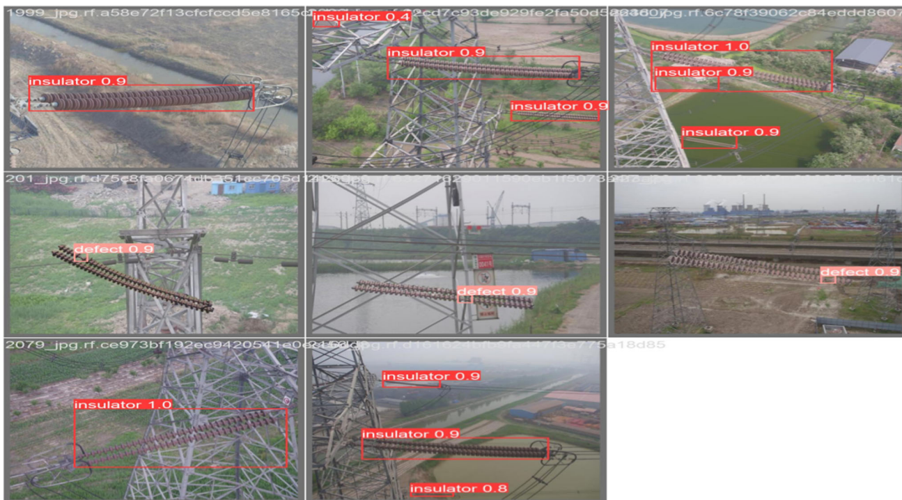
Fig. 9 Insulator defect detection results
