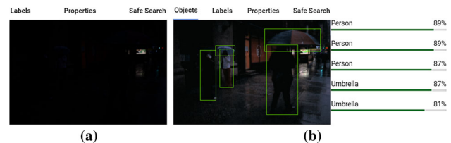
Fig. 11 Results of Google Cloud Vision API. a Recognizing result of low-light image; b recognizing result of our enhanced image
