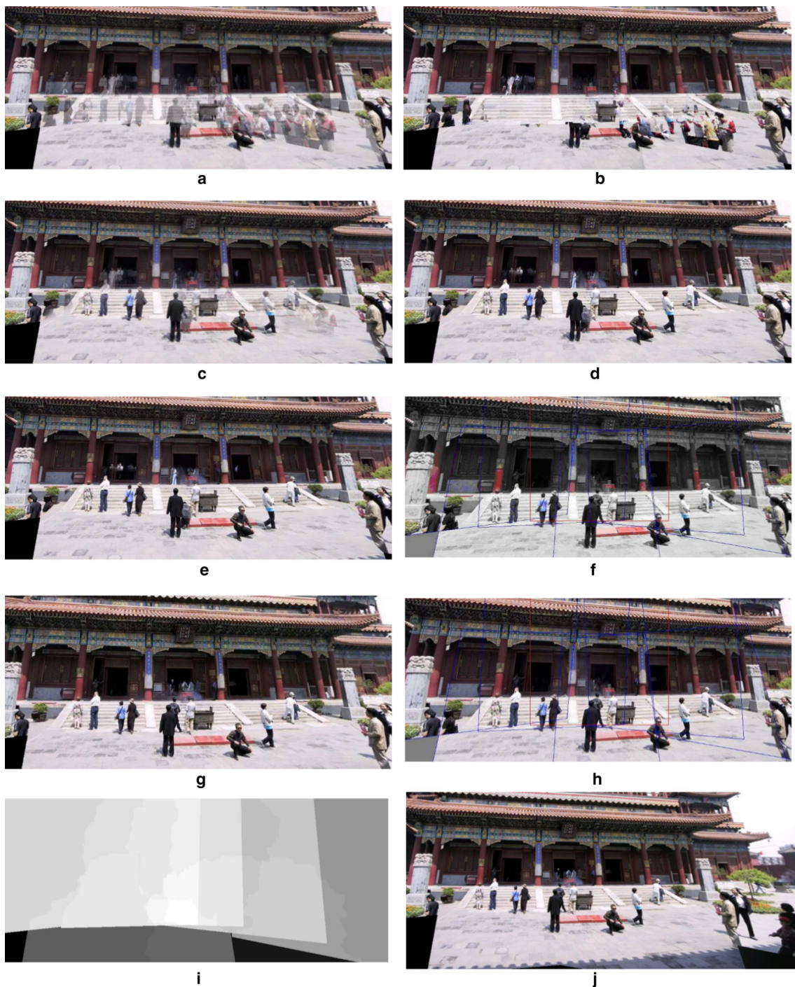
Fig. 16 Final composites computed by a variety of algorithms: a average. b median. c feathered average. d p -norm p = 10 . e Voronoi. f weighted ROD vertex cover with feathering. g graph cut seams with
