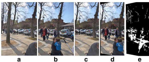
Fig. 4 a, b Images with OR [45]. c, d Overlap regions. e Calculated mask (images differences)
