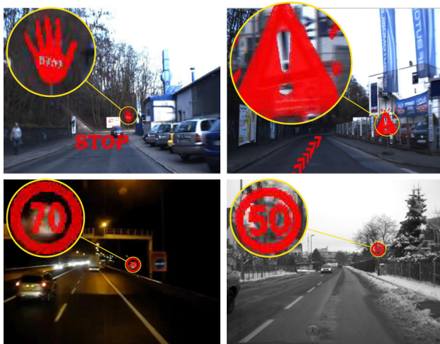
Fig. 4 Insertion of virtual 3D object sign in cloudy days, nighttime, sunny days and snow days
