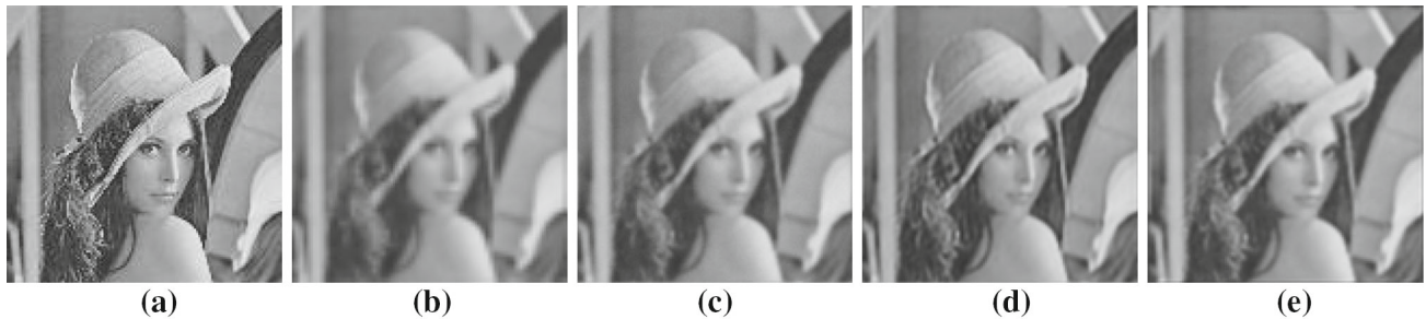
Fig. 4 Super-resolution case, Gaussian blur. a Original image, b one of the low-resolution images (interpolated), c CMA2-SR, d CMA2-C-SR, e bilateral shift-and-add method
