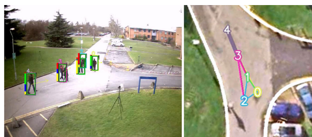
Fig. 6 Social forces representation. In the left image , we depict the output of our framework with IMM-PF SF. The four trackers are projected to the world plane through camera calibration ( right image ). The ( directed ) edges connect the trackers which interact with each other. Edges of same color correspond to the same tracker
