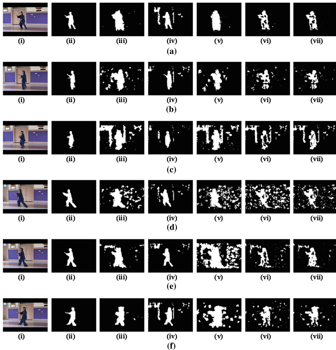
Fig. 6 Segmentation results for Taichi video sequence corresponding to a Frame 50, b frame 100, c frame 150, d frame 200, e frame 250, f frame 300 ( i Frame no. n , ii ground-truth segmented frame, iii segmented frame obtained by use of the proposed method, iv segmented
