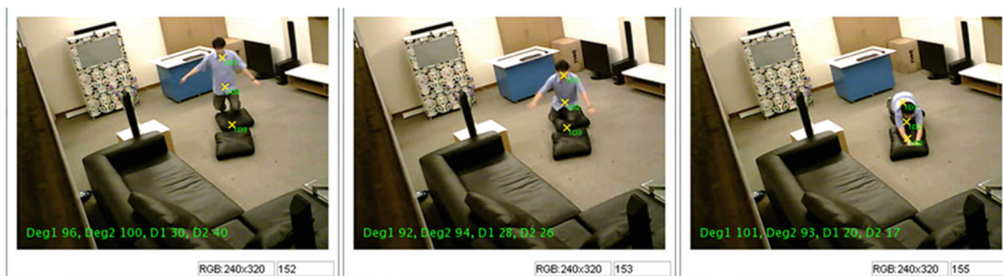
Fig. 9 Example of the no changes in the ratio of the distances ( \Delta p = 0 ) during a fall
