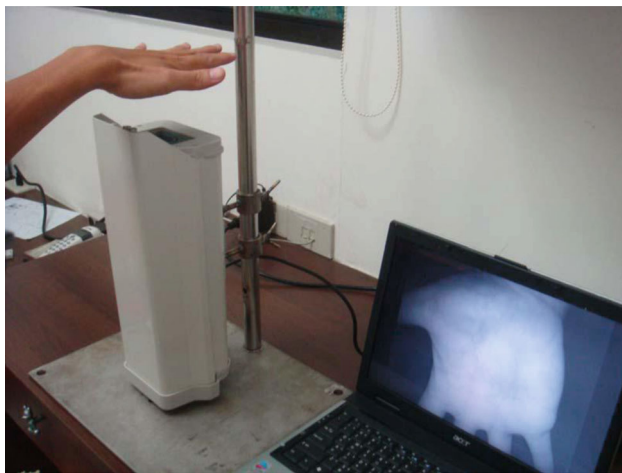
Fig. 2 Acquisition of palm vein images with a non-contact system
