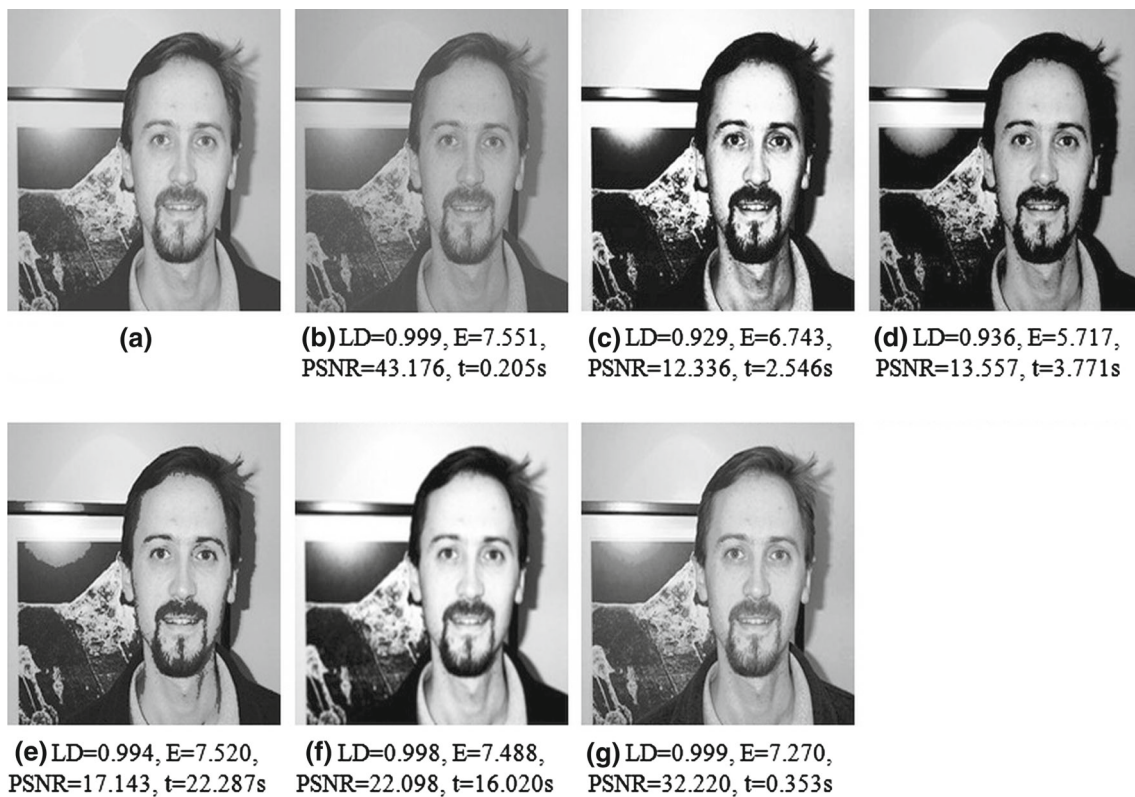
Fig. 8 Comparison of enhancement results a original ‘Man 1’ image, b proposed method, c NINT [1], d FOM [25], e FRB [13], f FL [30], g FHE [12]
