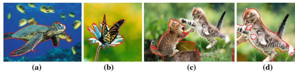
Fig. 7 Segmentation results. a Focused turtle and defocus background. b Focused butterfly together with flower, and defocused background. c Stationary non-blurred cat, ‘flying’ cat with a little blur and defocused background with more blur. d ‘Flying’ cat with a little blur and defocused background with more blur
