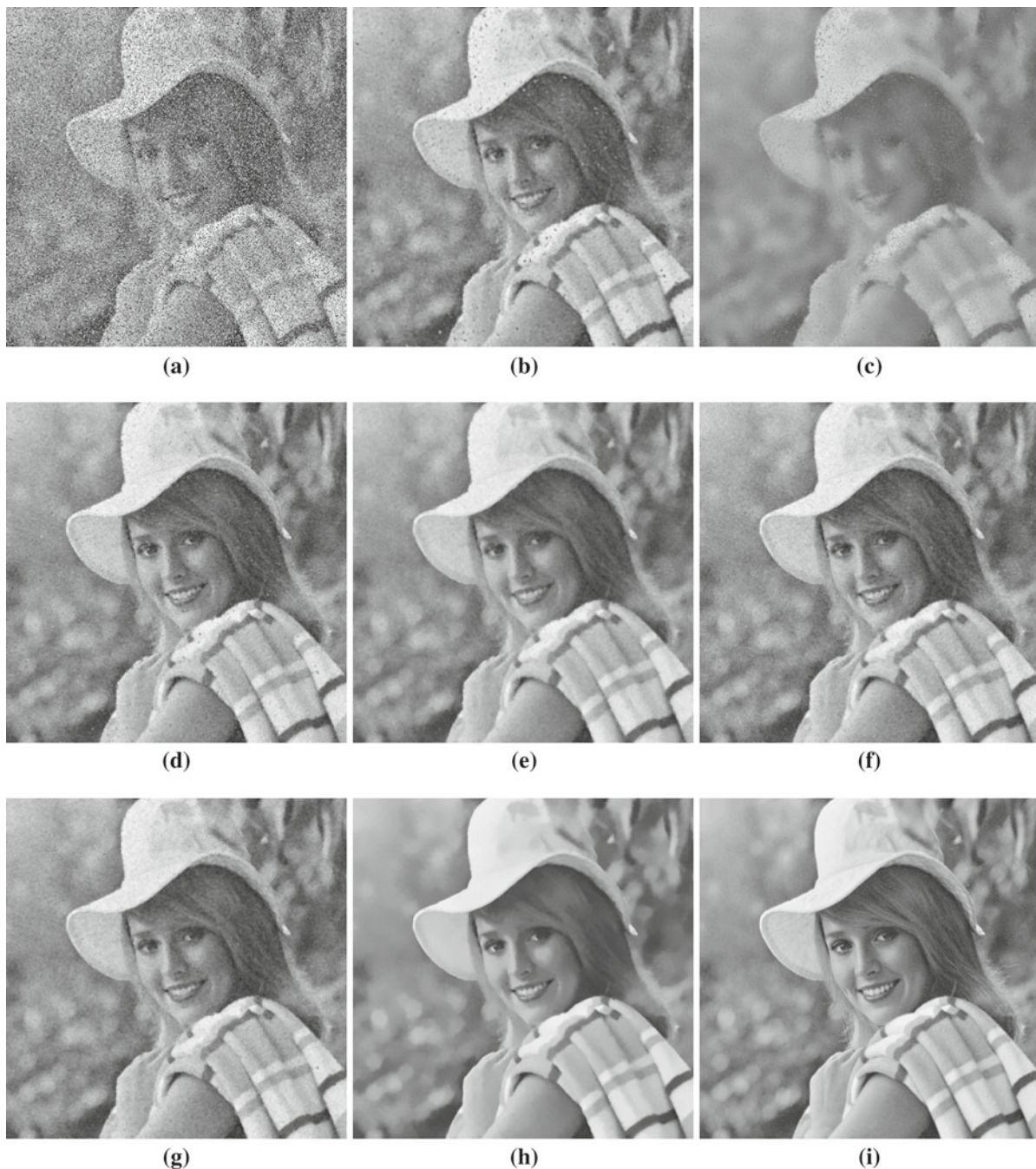
Fig. 4 Results of different filters in restoring mixed noise ( \sigma = 10 , p = 40\% ). a Noisy image, b SKR, c NLM, d GP, e Luo, f DWM, g CEF, h FWNLM and i the noise-free image
