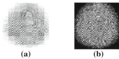
Fig. 6 a Acquired image. b Enhanced image after pre-processing
