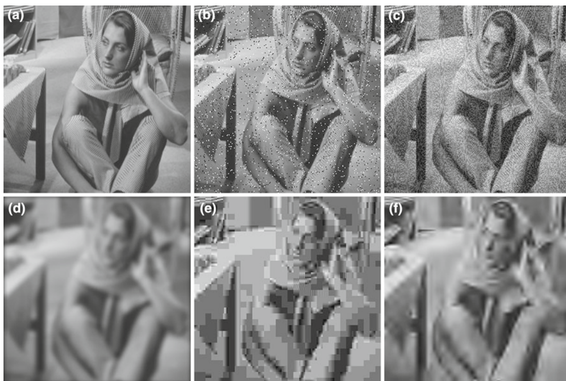
Fig. 2 Equal SSIM hypersphere: a original “Barbara” image; b 4% salt and pepper noise, SSIM = 0.4950; c 16.00\sigma Gaussian noise, SSIM = 0.4958; d 13 \times 13 Gaussian blur, SSIM = 0.4886; e 95% JPEG compression, SSIM = 0.4531; f 98% JPEG2000 compression, SSIM = 0.4980
