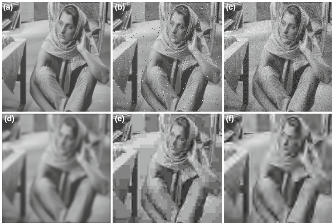
Fig. 1 Equal MSE hypersphere: a Original “Barbara” image; b 1.4% salt and pepper noise, MSE = 259.9516; c 11.35\sigma Gaussian noise, MSE = 258.6884; d 11 \times 11 Gaussian blur, MSE = 257.7267; e 90% JPEG compression, MSE = 259.6023; f 98% JPEG2000 compression, MSE = 270.2315
