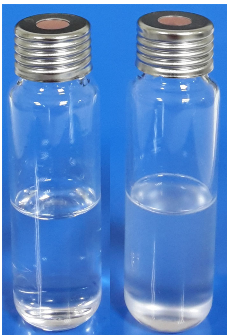
Fig. 10 Hydrolysis stability of p-NMA in a basic and b acidic medium at 80 °C (55 min)
