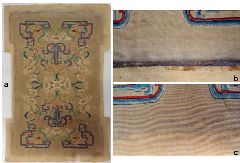
Fig. 8 Photographs of a whole contaminated window shade silk and contaminated partial side, b before cleaning, and c after cleaning
