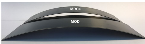
Fig. 14 Comparison between the curvature of the removed asymmetrical specimens [0_3]St for the standard (MRCC) and modified (MOD) cure cycle
