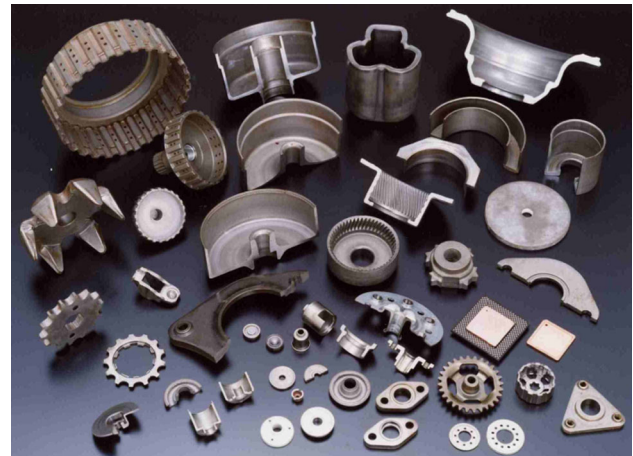
Fig. 4 Functional products formed by plate forging
