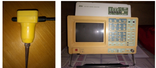
Fig. 1 Vibration pickup CB-30 and FFT analyzer AD-3523.
