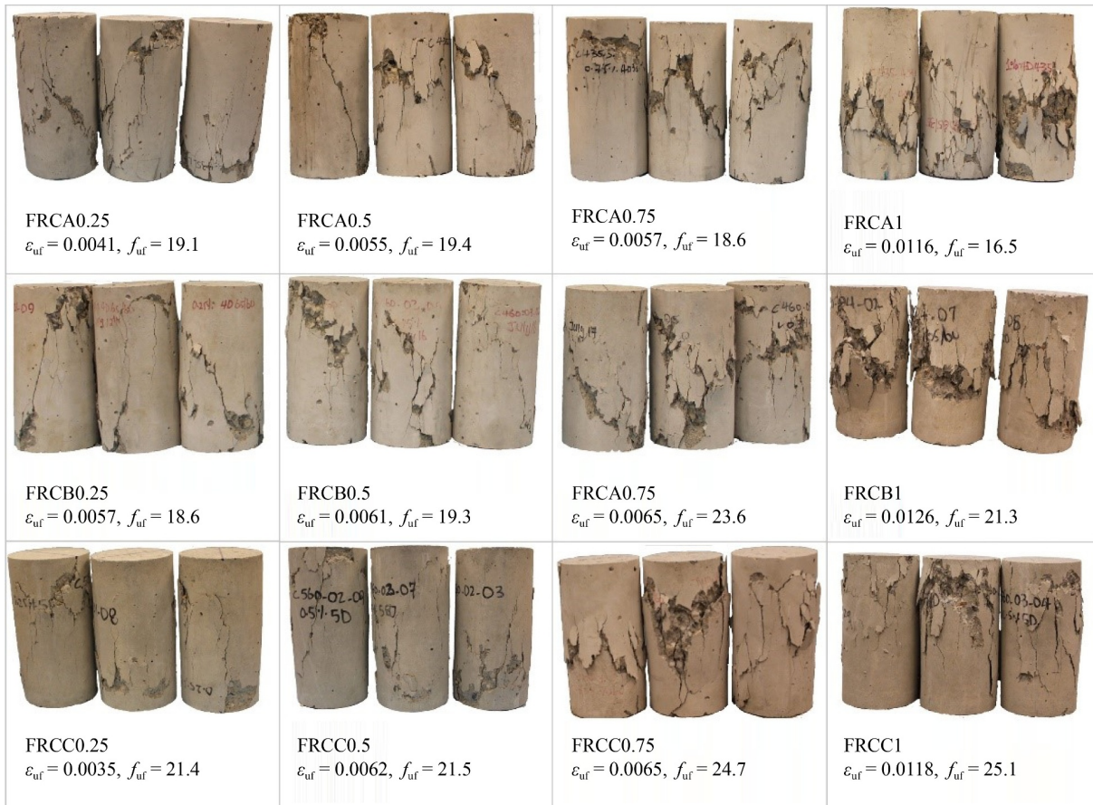
Fig. 4 Failure patterns of the specimens after compression test (the f_{uf} values are in MPa units).
