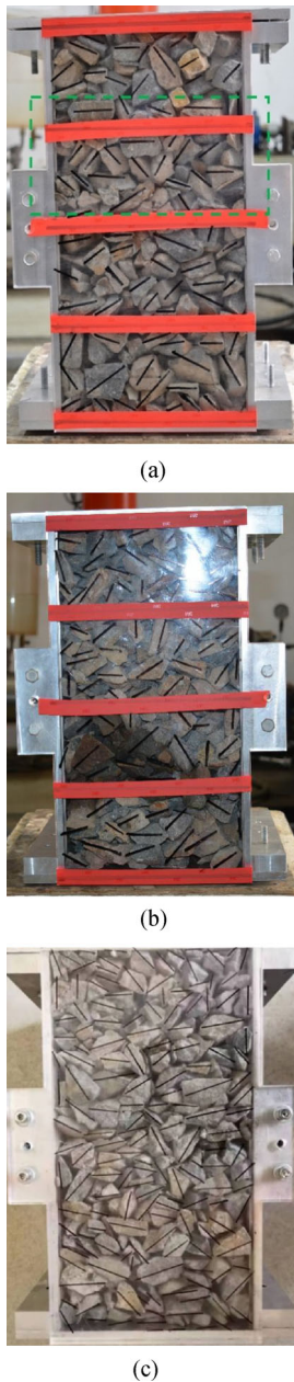
Fig. 4 Distribution of particle orientations: (a) low-density specimen; (b) medium-density specimen; (c) high-density specimen.
