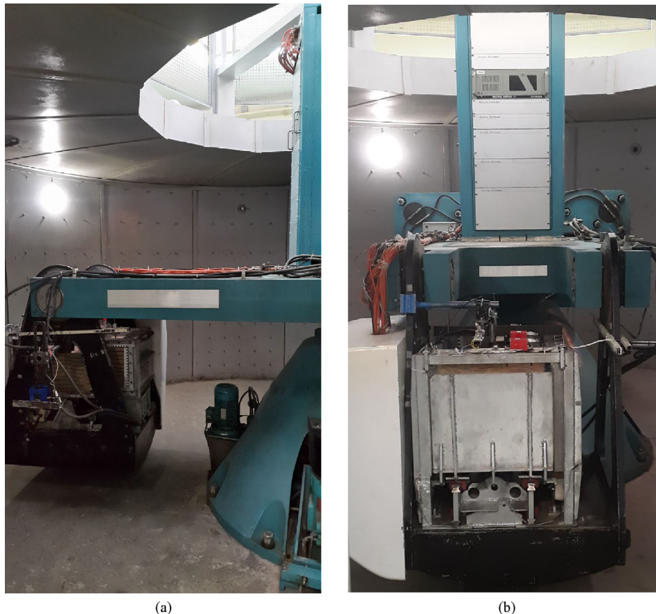
Fig. 5 The model installed in the centrifuge basket. (a) Side view; (b) front view.
