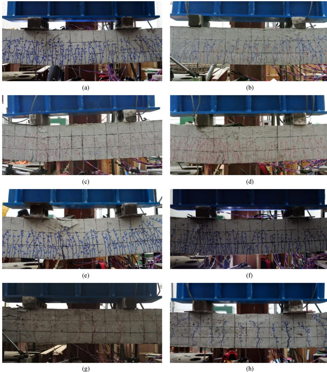
Fig. 9 Crack pattern in tested beams after ultimate failure. (a) Specimen N-1; (b) specimen N-2; (c) specimen S-1; (d) specimen S-2; (e) specimen T-1; (f) specimen T-2; (g) specimen RC-1; (h) specimen RC-2.
