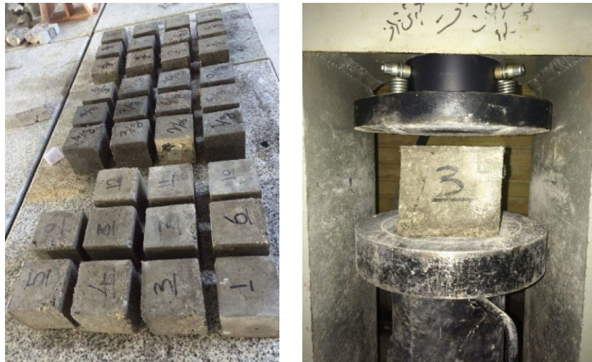
Fig. 1 Construction and testing process of the specimens
