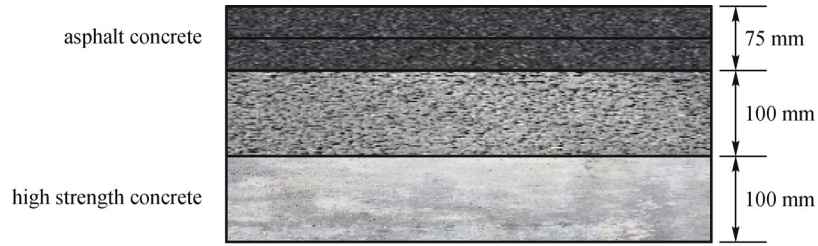
Fig. 16 Configuration of the innovative SHS multi-layer composite used in field blast test
