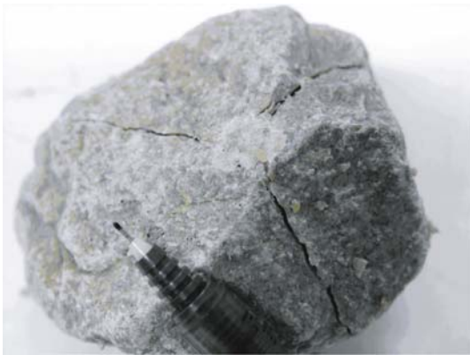
Fig. 39 Broken particle after test
