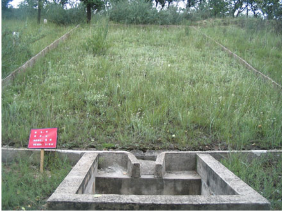
Fig. 6 Field plot for rainfall-runoff measurement in AJW
