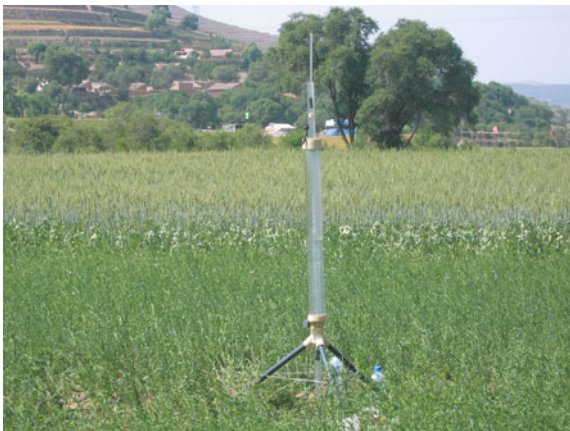
Fig. 4 A model of 2800K GP used for measuring Sol\_K in a farmland in AJW
