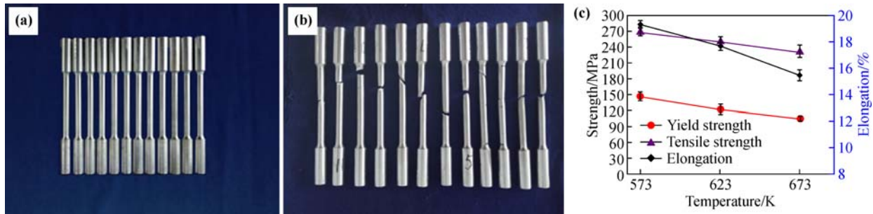
Fig. 6 The tensile samples (a) before and (b) after fracture. (c) The comparison of mechanical properties.
