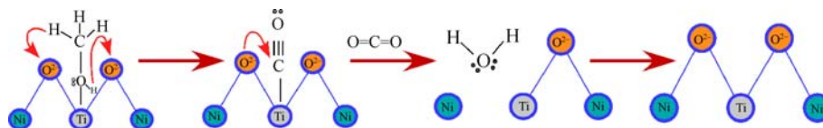
Fig. 9 Scheme demonstrating possible reactions through which the oxidation of methanol can occur in the presence of NiTiO 3 .
