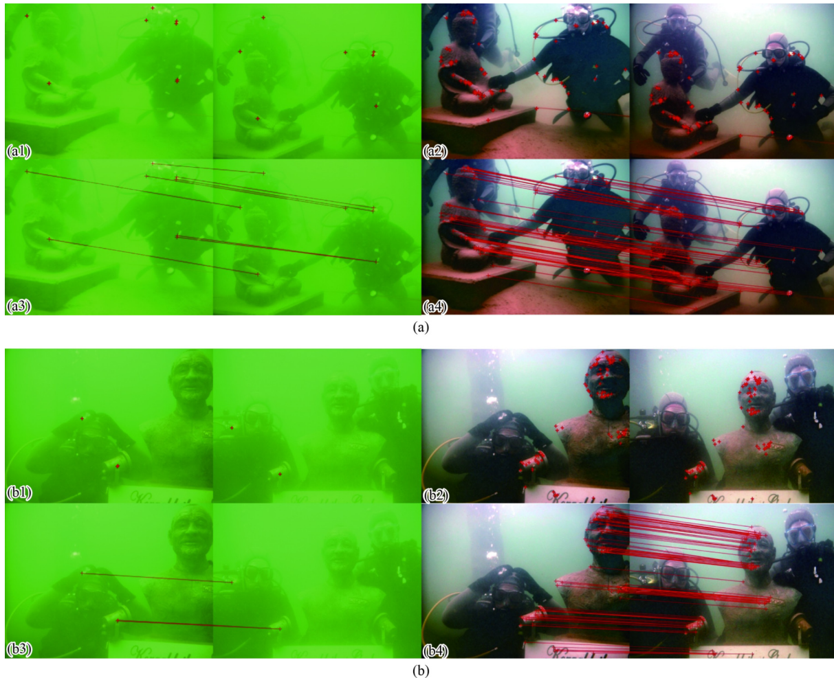
Fig. 13 Interest points detection and SIFT feature matching. For the left-side pair ((a1) and (a3), (b1) and (b3)), Harris corner detections only find 8 and 2 interest points that can be correctly matched when using SIFT features based on original image pairs. For the right-side pair ((a2), (a4), (b2), (b4)), there are 80 and 90 interest points found and correctly matched when using Harris corner detection and SIFT feature matching respectively based on dehazing image pairs. (a) The first pair of underwater images; (b) The second pair of underwater images
