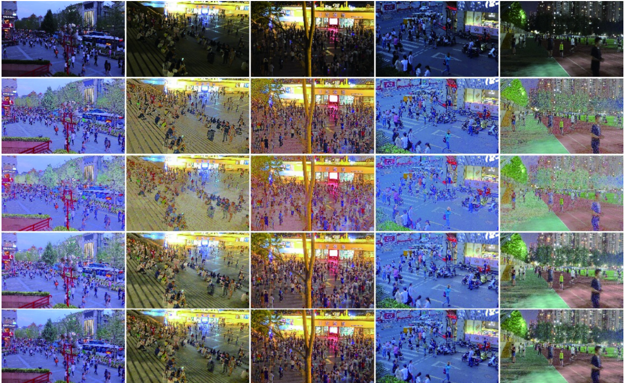
Fig. 4 The illumination enhanced results with different approaches. The first row is the initial images. The second row is the results with KinD [36]. The third row is the results with RetinexNet [37]. The fourth row is the results with LIMi [38]. The fifth row is the results with DUAL [35]
