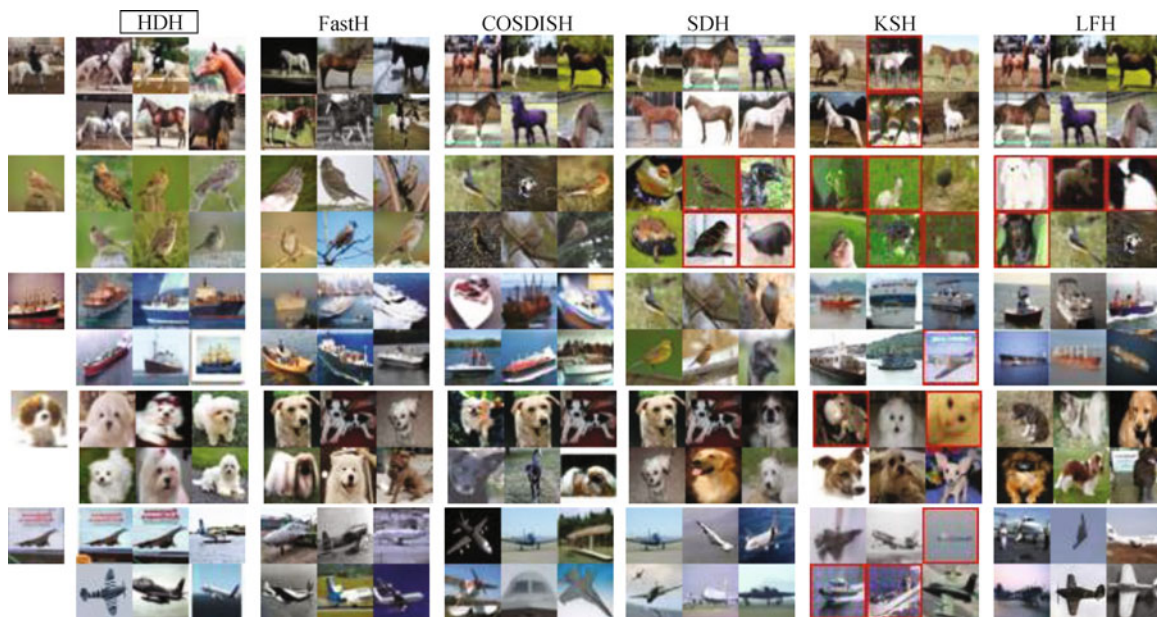
Fig. 6 Top six images of five queries are retrieved with different supervised hashing methods on the CIFAR10 dataset (The image on the first column is the query sample. From left to right are the retrieved results by HDH, FastH, COSDISH, SDH and LFH when 48-bit binary codes are used for search)
