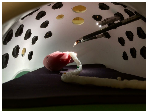
Fig. 2 View from inside the laparoscopic box trainer, with 3D-printed model secured and da Vinci ® Si robotic system docked
