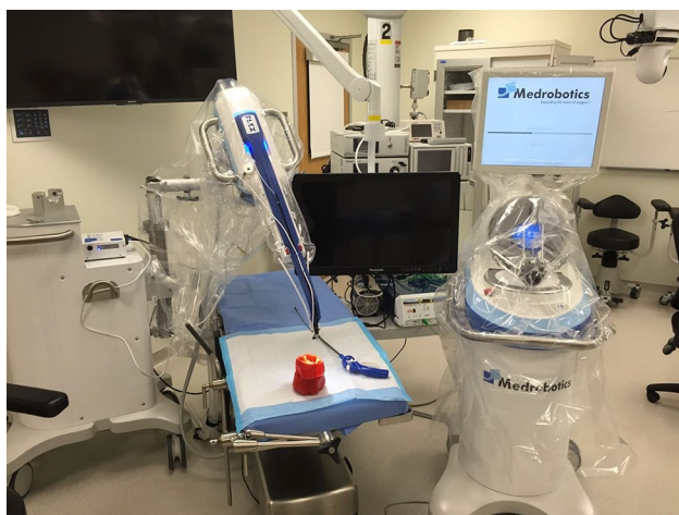
Fig. 1 Photo of components of Medrobotics Flex system. From left to right these comprise the robotic endoscope cart, the HD screen and the robotic control console
