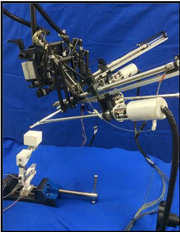
Fig. 1 A lateral view of IBIS VI, a 7 degree-of-freedom pneumatically driven surgical robot, during needle insertion
