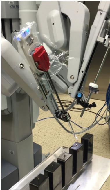
Fig. 2 Evaluation of haptic and tactile feedback of the daVinci system (Intuitive Surgical Inc.). The surgical system is tested using a standardized investigation procedure
