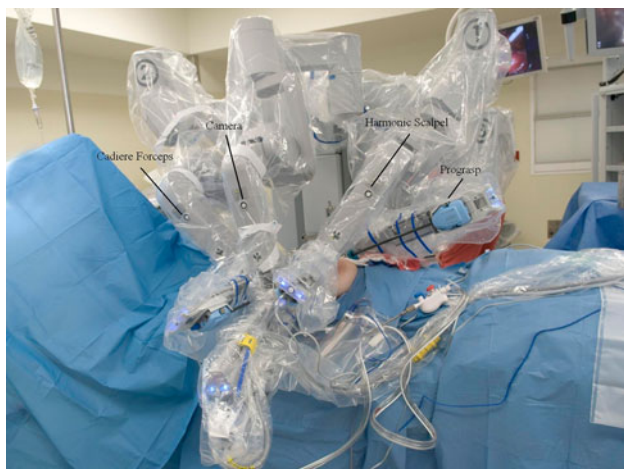
Fig. 1 Intraoperative photo showing the position of the robotic instruments for transaxillary thyroidectomy
