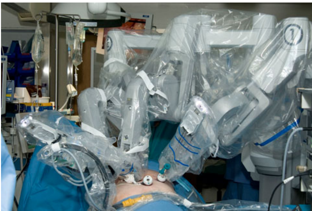
Fig. 6 Positioning of the robot for a left lateral transabdominal adrenalectomy. In this procedure there is an additional port for the first assistant
