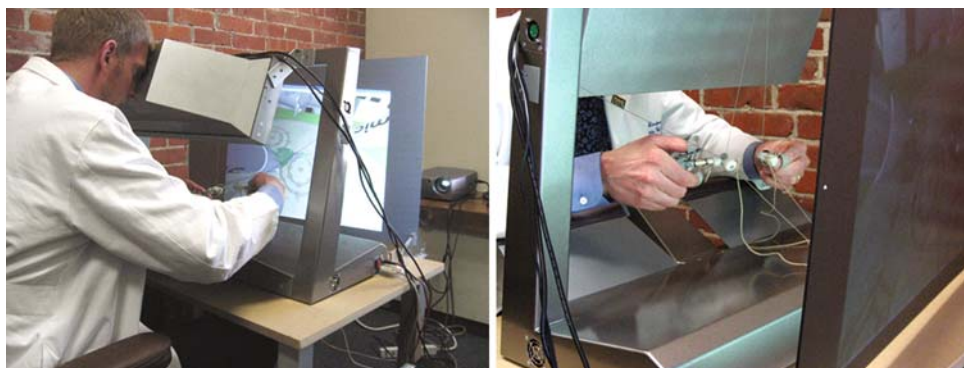
Fig. 1 Virtual-reality 3D dV-Trainer simulator platform
