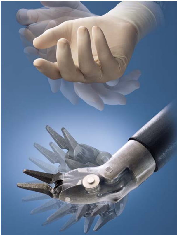
Fig. 3 EndoWrist robotic instrument (photo courtesy of Intuitive Surgical)
