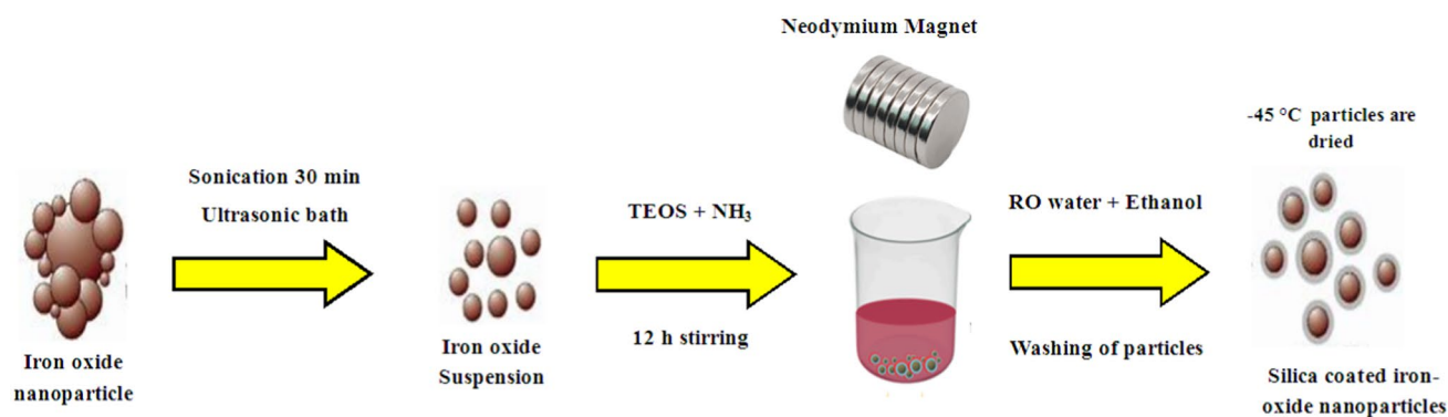
Fig. 1 Flowchart demonstrating the process for the synthesis of Si/Fe 3 O 4 nanoparticles
