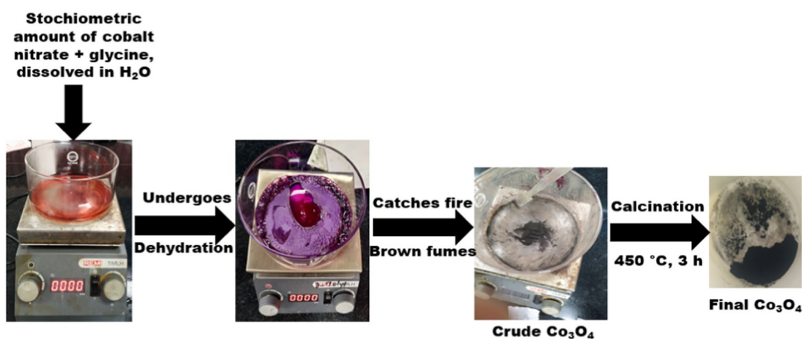
Fig. 1 Schematic representation of \text{Co}_3\text{O}_4 nanopowder synthesis via autocombustion method
