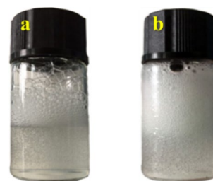
Fig. 5 Freezing resistance tests of AFFF concentrate ( a : Sample before treatment; b : Sample after treatment)
