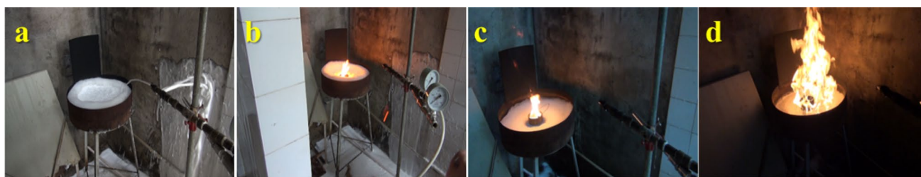
Fig. 4 Pool fire resistance tests of 6% AFFF diluent ( a : Continue spraying the 6% AFFF for 3 min; b : Ignite the fuel in the burning tank; c : After 12 min of fire resistance; and d : After 18 min of fire resistance)
