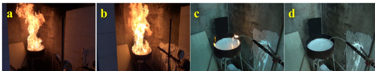
Fig. 3 Pool fire extinguishment of 6% AFFF diluent (a: Pre-combustion for 1 min; b: 52", a quantity amount of foam was added; c: Extinguishing fire; and d: 1'50", completely extinguished)
