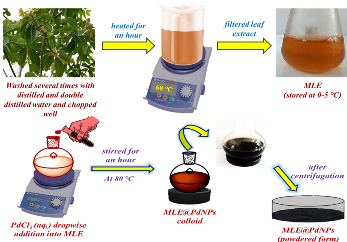
Fig. 2 Systematic representation of preparation of Mahua leaves extract (MLE) and synthesis of MLE@PdNPs at 80 °C
