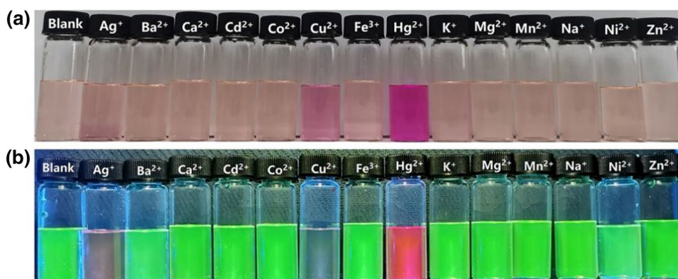
Fig. 2 a The color changes of probe RB (10 \mu\text{M} ) with different metal ions (100 \mu\text{M} ) in the mixture solution EtOH/ \text{H}_2\text{O} (V/V = 1:1) under day light. b The color changes of probe RB (10 \mu\text{M} ) with different metal ions (100 \mu\text{M} ) in the mixture solution EtOH/ \text{H}_2\text{O} (V/V = 1:1) under 365 nm UV-lamp
