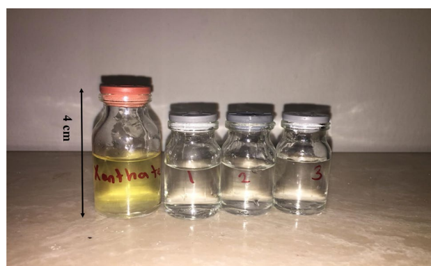
Fig. 11 Initial xanthate solution and the clean supernatants obtained with copper electrodes (pH 9 and 0.6 A and desirability = 1)
