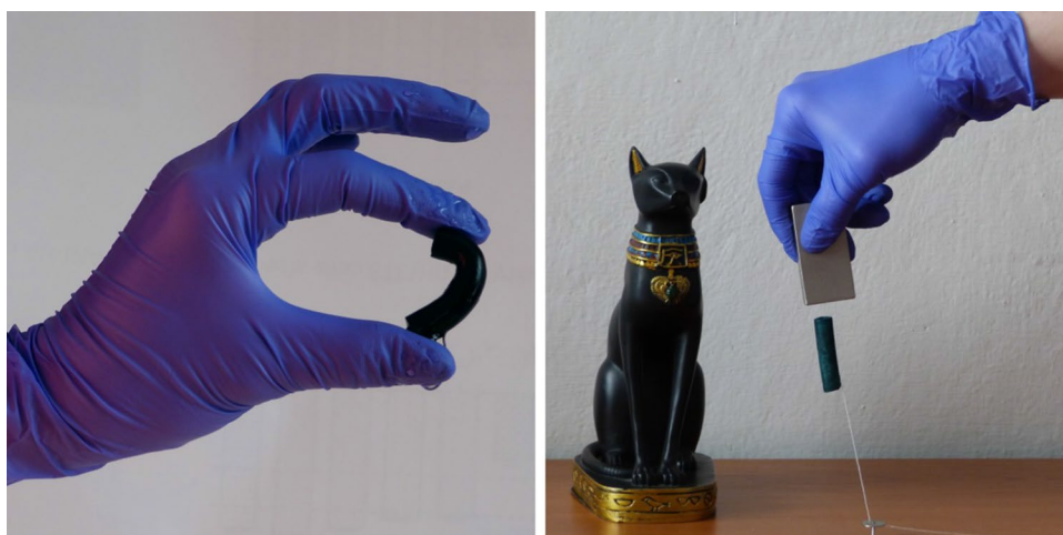
Fig. 19 Illustration of a conducting polymer cryogel containing ferrite particles (left). Magnetic aerogel obtained after freeze-drying is attracted to a magnet (right) (Islam Minisy, unpublished results)
