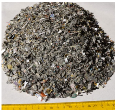
Fig. 2 Crushed PCBs of mobile phones—8 mm
