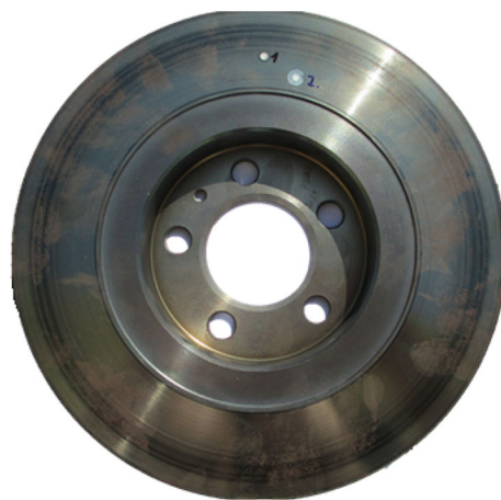
Fig. 2 The brake disc after GDOES profile analysis
