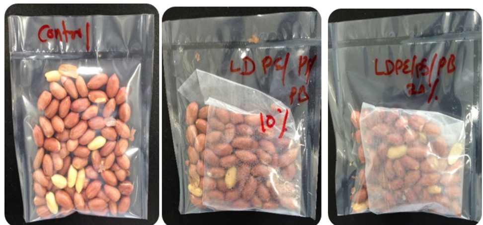
Fig. 1 Storage test of oxygen scavenging packaging containing LDPE/PSN films (10 and 20%) and roasted peanut samples
