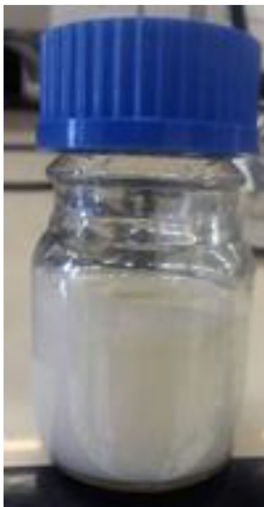
Fig. 6 Visual appearance of optically translucent and stable nanoemulsion (containing 7 wt% orange oil, 3 wt% sunflower oil, 2 wt% Tween 80 and 88 wt% aqueous phase prepared at a stirring speed of 500 rpm at 35 °C at the first step and 10 min' sonication at the final step)
